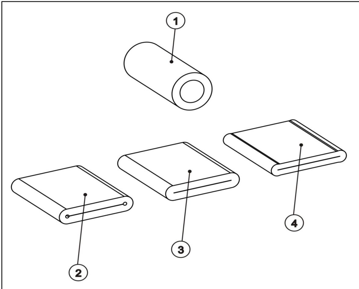
*Fig. 3: Squeezing the hose*
